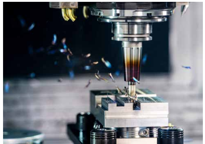
Full-slot milling with CELSIO heat shrinking toolholder
