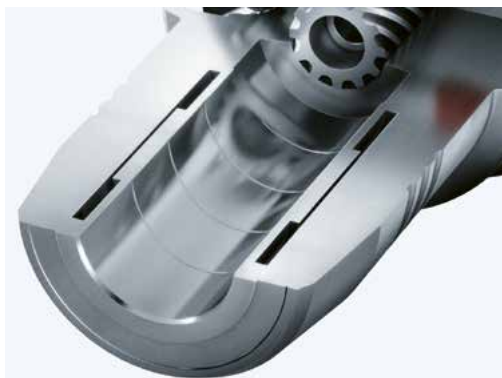
Dirt grooves for reliable torque transmission
