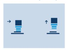
A slight pushing movement releases the pillars from the surface and the workpiece is gently detached.
