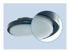
The ADHESO gripper is based on the principle of dry adhesion, which is based on intermolecular forces ("Van der Waals forces"). The pillar structure shown here maximizes contact with the surface. As a result, the gripper does not require an external power supply and can reliably grip a wide range of different materials.
