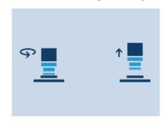
A slight rotary movement releases the pillars from the surface and the workpiece is gently detached.
