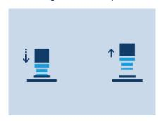
Due to excess pressure, the pillars buckle in on themselves and release the contact to the workpiece surface (only possible with the 700  $\mu m$  structure).
