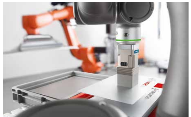
Handling of sheet metal
