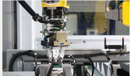
Change systems & feed-through modules
