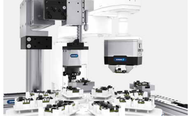
Handling of electronic assembly groups with a SCARA robot
