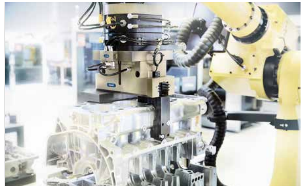
Handling of motor blocks
