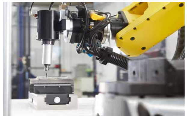
Controlling electric deburring spindle RCE
