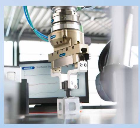
Depending on the workpieces and processes, various testing and measuring procedures can be automated. Quality inspection and quality assurance serve to ensure product quality during production. Handling and sensor components enable automated quality inspection and support documentation of measuring and inspection values.
