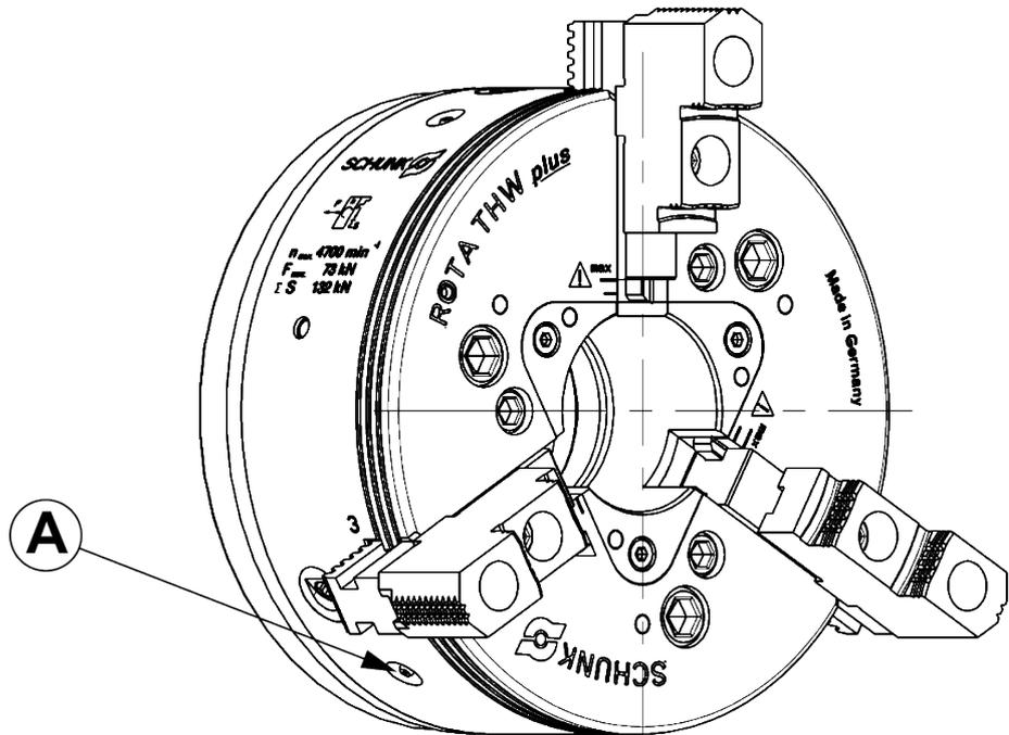
The following number of grease gun strokes must be applied to the chuck at each of the 3 lubrication points:
