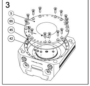
Remove screws (65) and pull out cover (5) together with 0-ring (45) and flat gaskets (48) out of the housing. To do this, screw two screws into the threaded holes as an extraction tool
