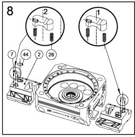
Pull the base jaws (2) out of the housing.
