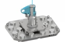
Clamping of landing gear component: shackle
