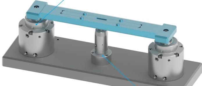
Micro adjustment and spring adjuster can be used in combination.
