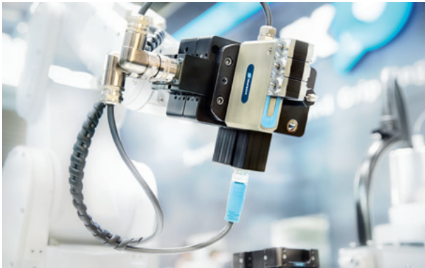
EGM: Handling of motors
