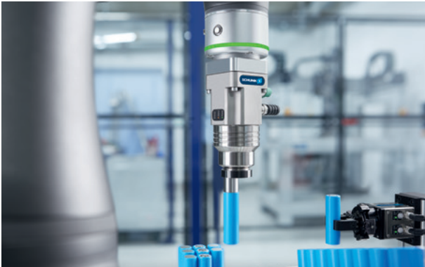
EMH: Handling of battery round cells
