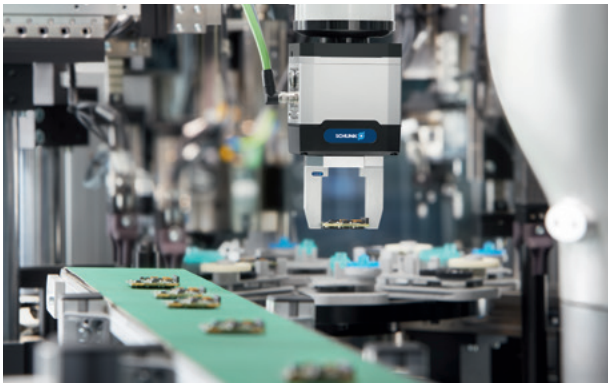
EGK: Handling printed circuit boards
