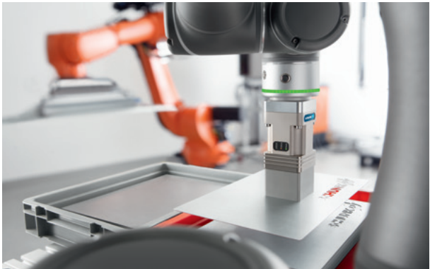
EMH: Handling of sheet metal
