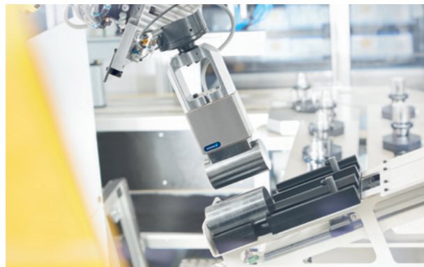
Pick & place with magnetic grippers
