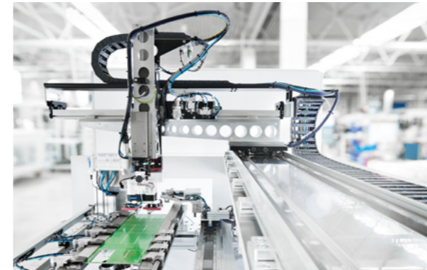
Separating circuit boards
