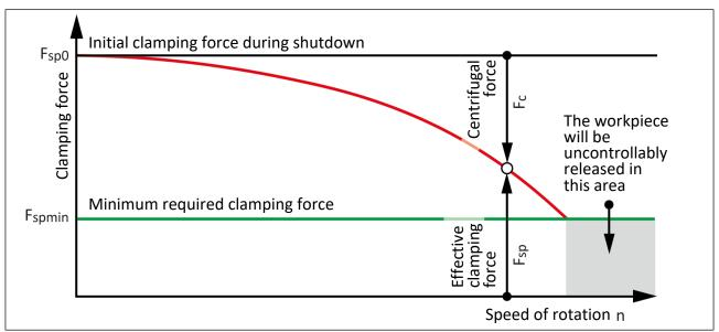
Reduction in effective clamping force by the magnitude of the total centrifugal force, for gripping from the outside inwards.
