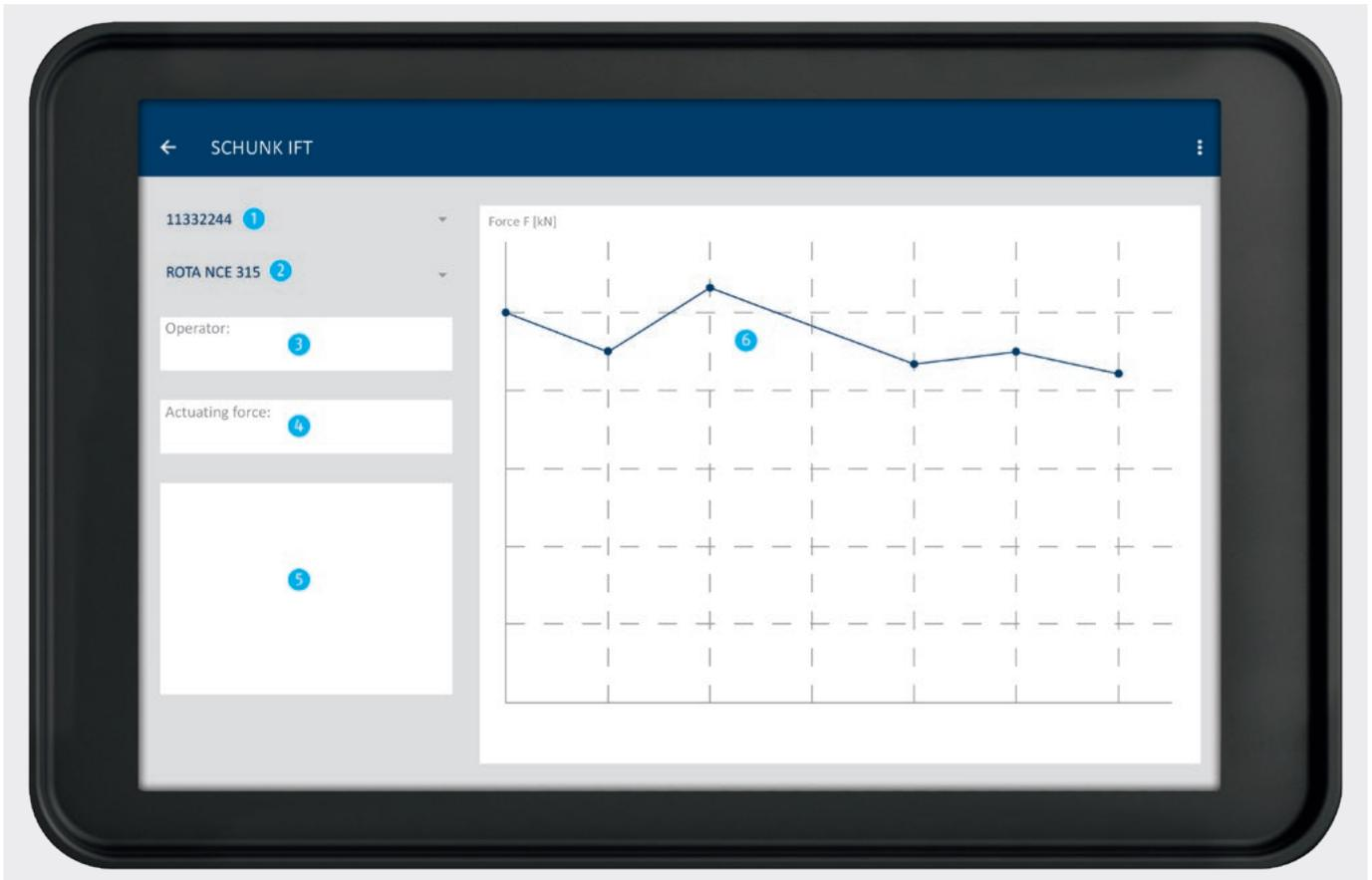
The integrated database allows access to stored measured values. Each clamping device is stored in a machine-related way. This allows the measured values to be visualized at any time via the app.
