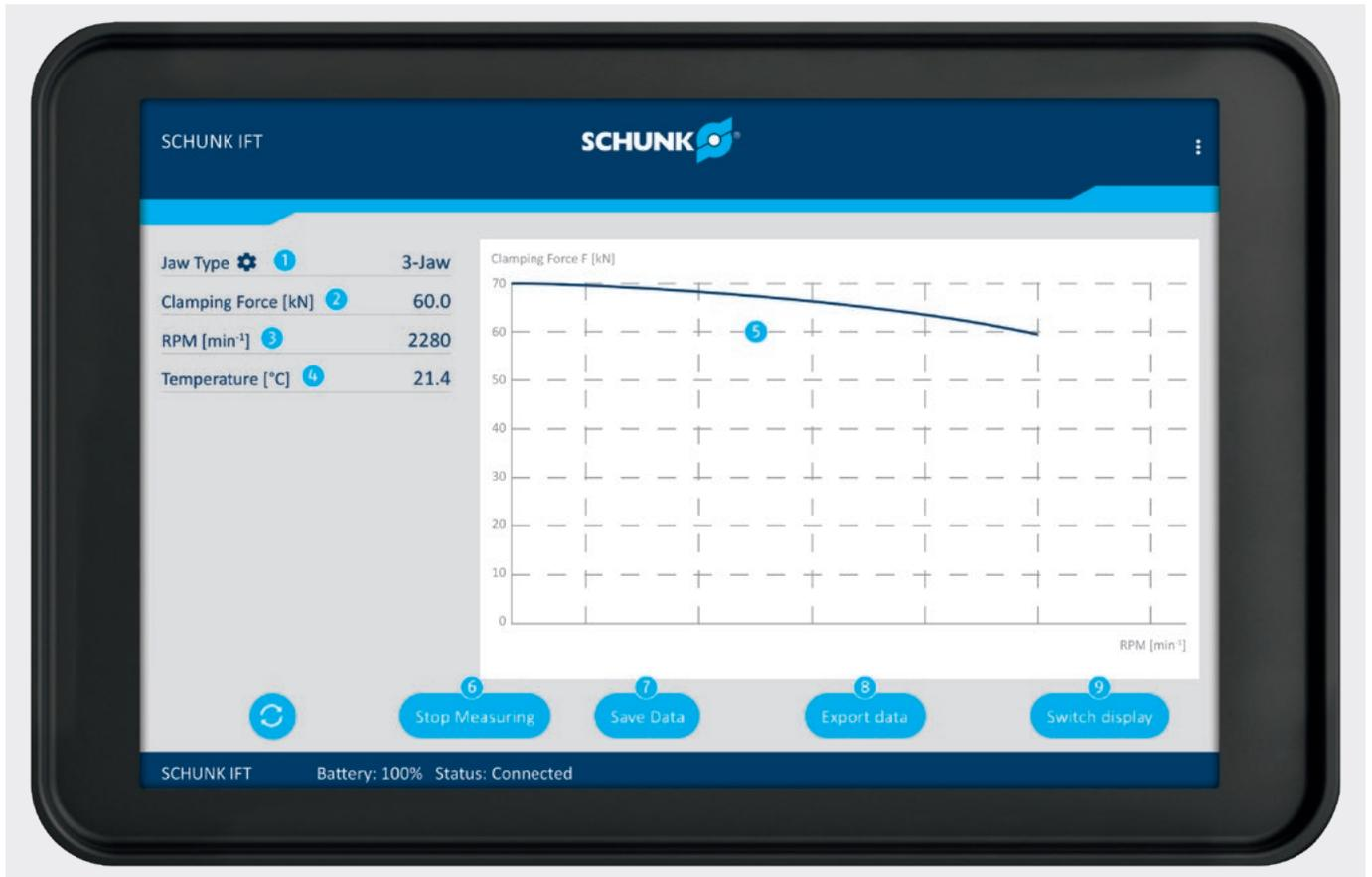
A particularly user-friendly operator interface enables all users to operate the clamping force tester intuitively. Depending on the application, the app offers an optionally adapted interface. An example of this is the high-resolution clamping force/speed diagram for dynamic clamping force measurement.
