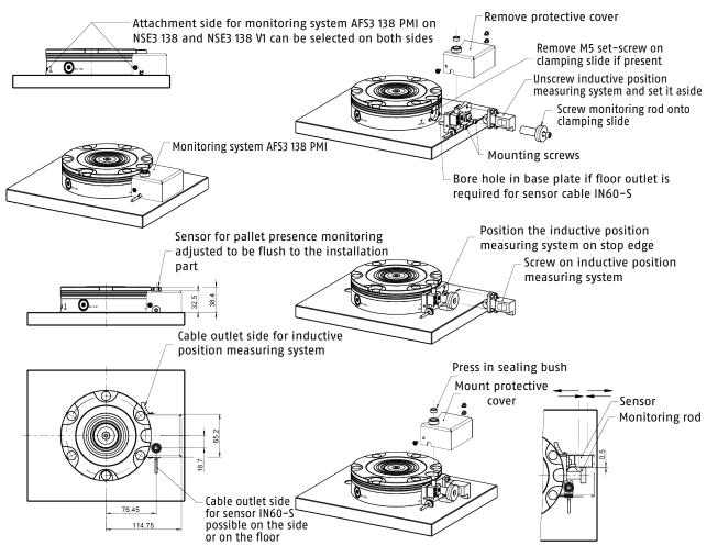
The unit is installed to a VERO-S NSE3 according to the following assembly steps
