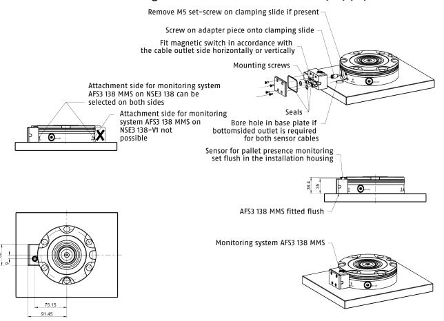
The unit is installed to a VERO-S NSE3 quick-change pallet system according to the following assembly steps
