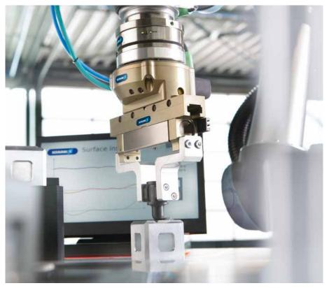
Depending on the workpieces and processes, various testing and measuring procedures can be automated. Quality inspection and quality assurance serve to ensure product quality during production. Handling and sensor components enable automated quality inspection and support documentation of measuring and inspection values.
