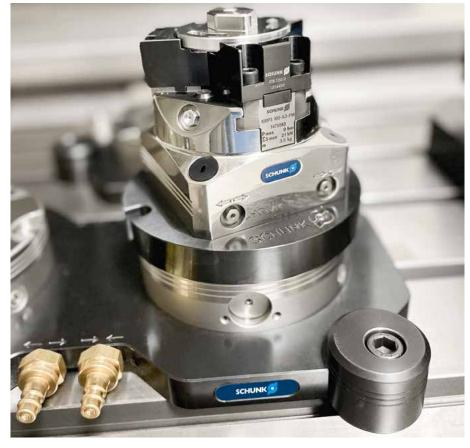
The TANDEM3 modular system, unique in its range of variants, is growing even more. In step one of the new generation, the 2-jaw clamping fore blocks were replaced and equipped with even more technical refinements: an absolutely fresh SCHUNK innovation being added - the TANDEM3 modular system has been extended by 3-jaw clamping force blocks.
