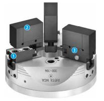
Supporting jaw With double jaw mounting for 0.D. and I.D. clamping
